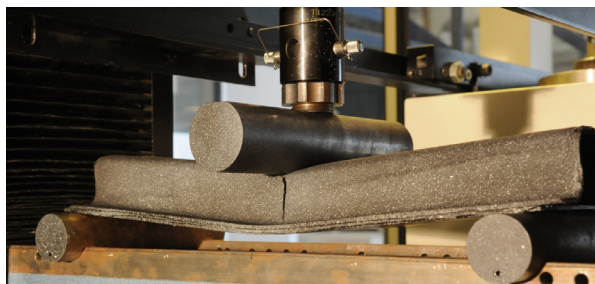
Figure 5: 3-point Flexure Test Setup
